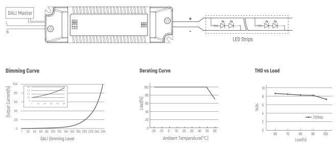
Note: For capacitive load, the larger inrush current will reduce the service life of the electrolytic capacitor. Before using this product, please contact the relevant technical personnel to match and verify.
