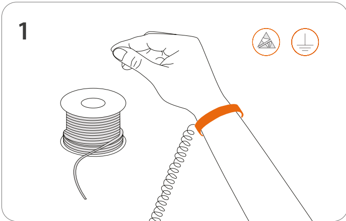
1 Work in an ESD protected environment. Make use of an anti-static strap.
